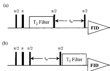
**Figure 1.** RNP experiment: (a) pulse sequence for RNP and (b) pulse sequence for referencing. The  $180^\circ$  pulse, which is optional, is used to refocus chemical shift during the preparation period of the NOE experiment. Typical NOESY phase cycle is applied.
